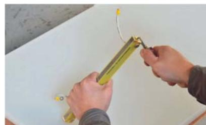
6. Put the other side of heating wire into another side fastener groove, then screw the remaining heating wire by the special tool.
