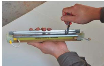
2. Remove the pressing stick from the complete sealing bar by cross screwdriver, then remove the stainless steel base (gas bag base).
