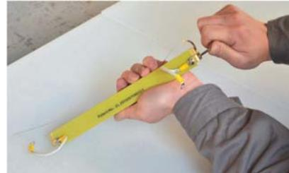
5. Put one side of a new heating wire into the fastener groove and tighten it by spanner.
