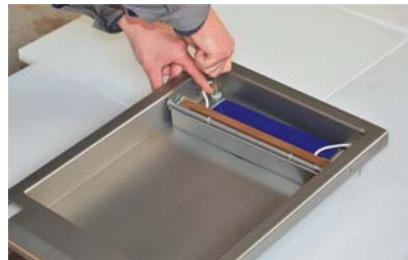
1. Disconnect the cable from the pin, then pick the complete sealing bar up from the vacuum chamber.
