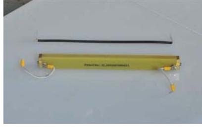
4. Remove the forcing screws from the two sides of sealing bar by Allen key, then take out the heating wire.
